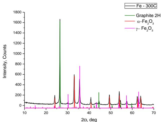
Figure 6. The XRD spectrum of material calcinated at 300 °C.
