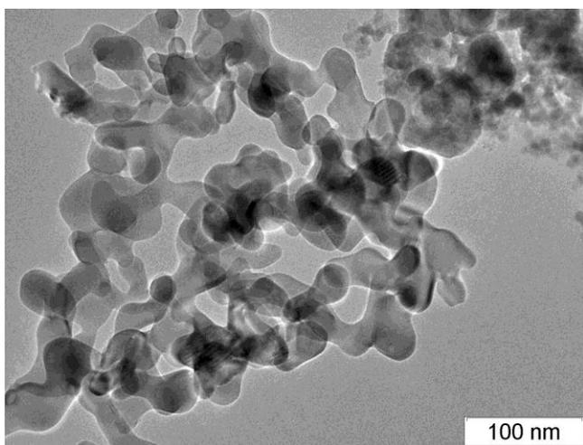
Figure 2. The morphology of the material calcined at 400 °C.
