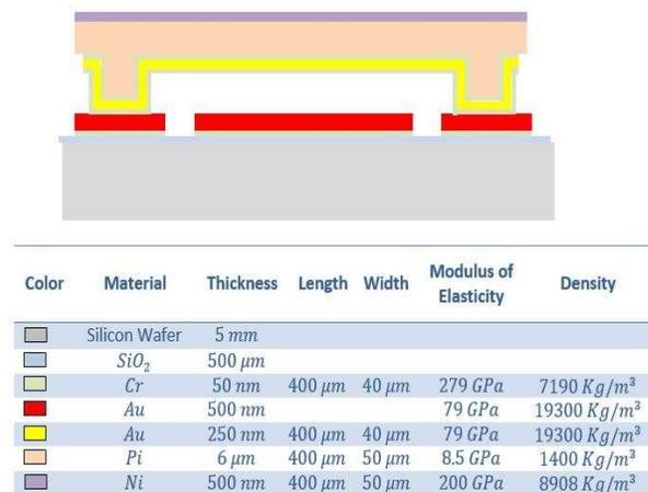
Figure 3. Cross sectional view of the fabricated microbeam.
