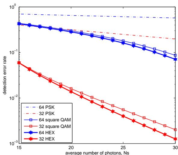
Figure 4. Detection error rate for  $M = 32$  and  $M = 64$
