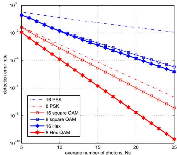
Figure 3. Detection error rate for  $M = 8$  and  $M = 16$
