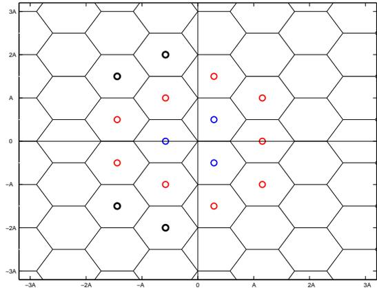
Figure 2. States set for 16-ary hexagonal QAM
