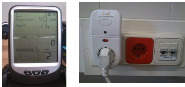
Figure 3. Smart meter (Current Cost) and his wireless connection
