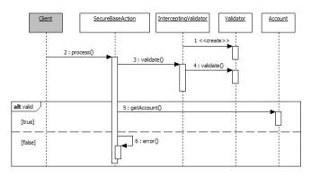
Figure 6. Intercepting Validator sequence diagram
