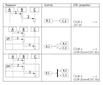
From the example of UML sequence diagram given in Figure 6, four LTL properties are generated. Table II lists them. These capture the cause-effect relations of every pair of methods found in the UML sequence diagram.
