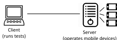
Figure 1. Client-server interaction in a mobile testing environment.
