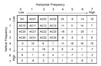
Figure 1. Generation of Low-frequency DCT coefficients (used as phase information)
