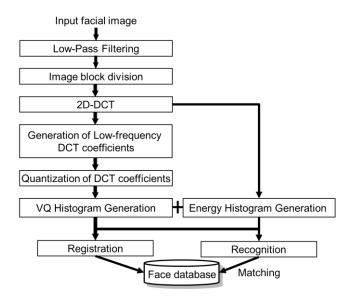
Figure 2. Face recognition process using combined histogram-based features.
