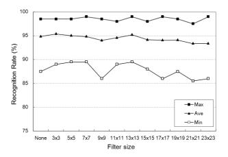
Figure 5. Recognition rate as a function of filter size (image block size is 8x8 here)
