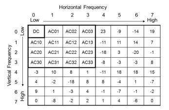
Figure 3. Low-frequency DCT coefficients for energy histogram.
