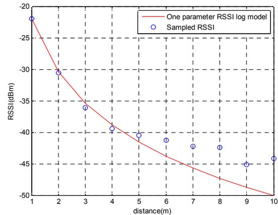
Figure 1. RSSI attenuation according to the elapsed distance.
