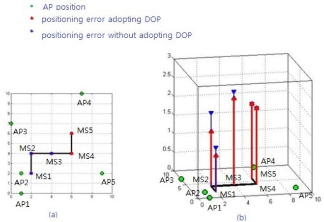
Figure 5. Experiment result comparison: (a) MS path and AP position distribution. (b) Comparison of positioning error adopting DOP and positioning error without adopting DOP.
