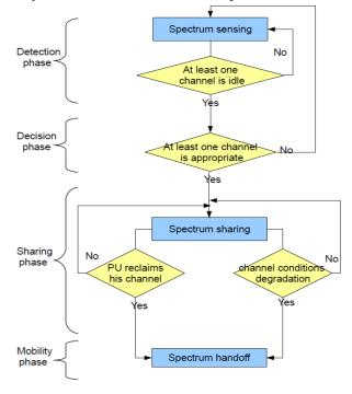
Figure 2. State diagram of cognitive radio node behavior
