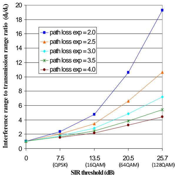
Figure 3: Min. relative distance separation vs SIR thresholds
