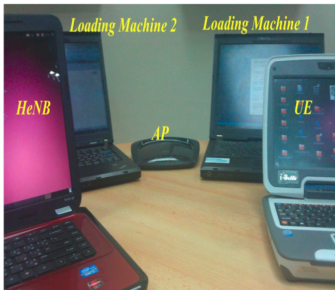
Fig. 8. Real setup of the LTE/WiFi Multi-RAT prototype.
