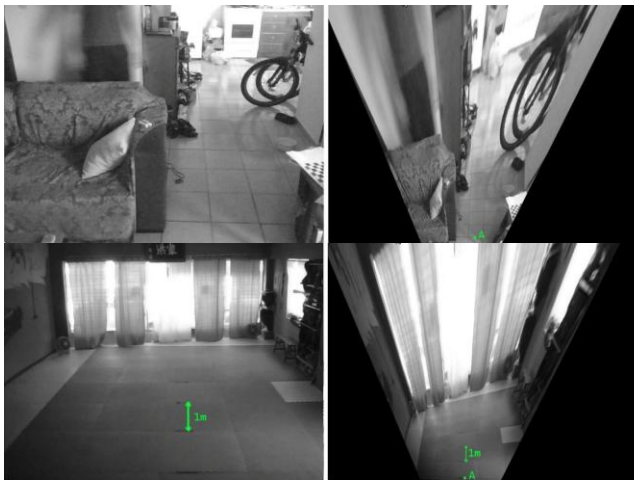
Figure 4: Input images and their inverse perspective transformation mappings
