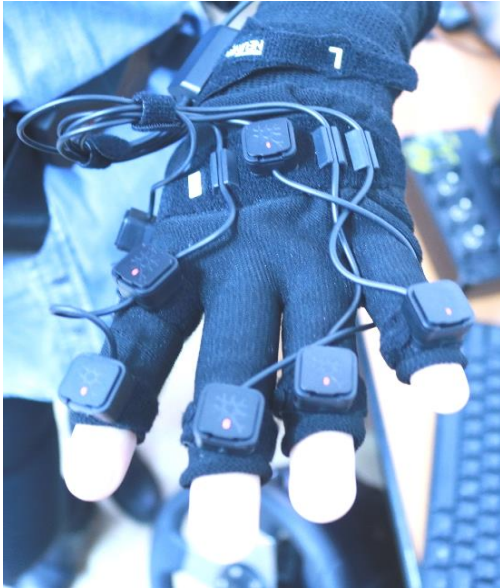
Figure 3. Perception Neuron inertial glove, sensing elements and connections.
