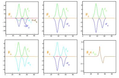
Figure 2. The plots of production rates  $F_i$  and reaction rates  $r_i$ . All production rates except  $F_6$  show an approach to equilibrium. The horizontal axes show the time in seconds, the vertical axes:  $F_i$  and  $r_i$  in  $s^{-1}$ .
