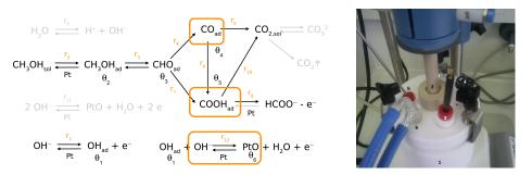
Figure 1. On the left: the chemical reactions network, the orange boxes show the reactions potentially responsible for the hysteresis effect on the CV plot. On the right: the experimental setup, consisting of a teflon cell (1) under deep vacuum, the rotating working electrode (2), the counter electrode (3), the reference electrode (4), the temperature sensor (5) and argon blow supply (6).
