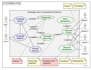
Figure 6. Use-case diagram of the knowledge-centric computation architecture: Two major use-case groups with four creator roles.
