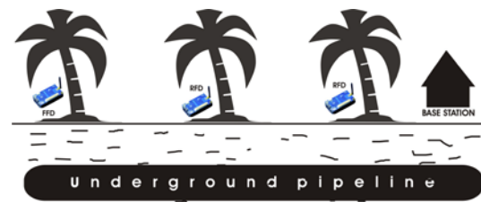
Figure 8. Cluster of FF and RF Devices placed on trees along the path of underground pipeline. Cluster will be repeated along total distance of underground pipeline
