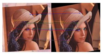
Figure 7. Descriptor extraction and matching using our improved algorithm in MatLAB
