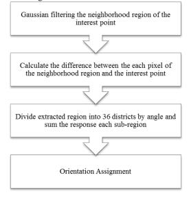
Figure 4. The modified algorithm flow chart
