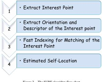
Figure 2. The SURF algorithm flow chart
