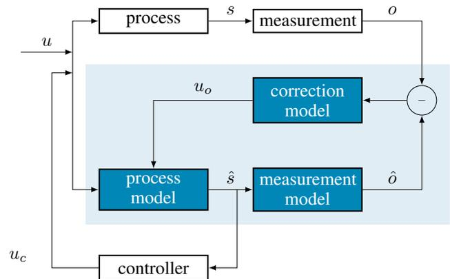
Figure 1. Components of the observer (blue) in parallel to the process.
