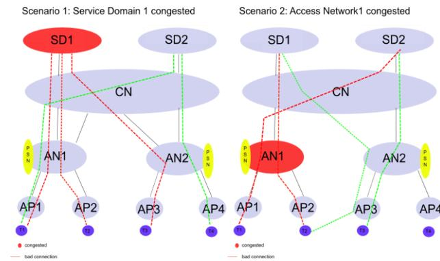
Figure 3. Different modes of failure in a multi-operator, multi-access-technology environment.
