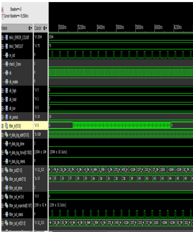
Figure 15. Pre-Synthesis Waveform of DDC
