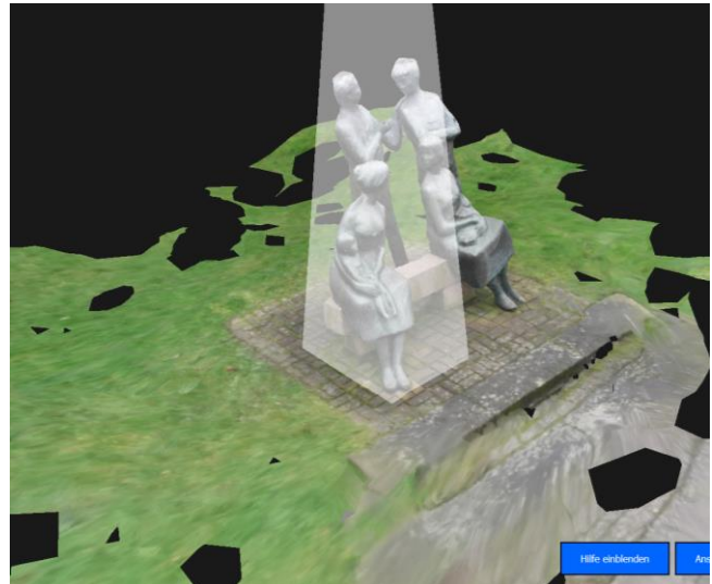
Figure 15. Screenshot of the 3D object in cutting mode. Also parts of a larger 3D object may be cut out using 3DEdit and use, e.g., in InfoGrid.
