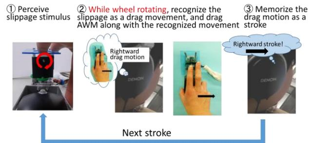
Figure 6. “While-perceiving-go strategy” for stroke presentation. The step ② in this figure can be regarded as an on-line integration of the steps ② and ③ in Figure 4, i.e., the “after-recognition-go strategy.”
