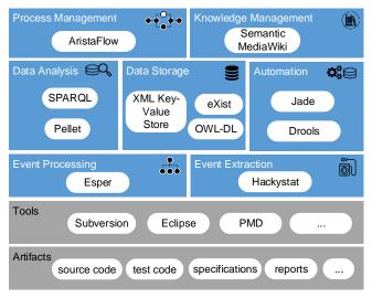
Figure 4. Framework Implementation for Software Engineering.
