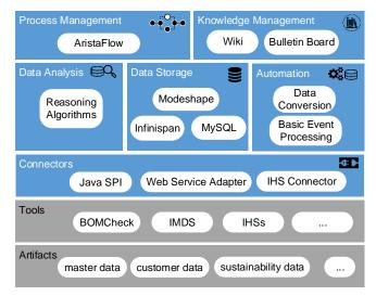
Figure 6. Framework Implementation for Supply Chain Data Collection.
