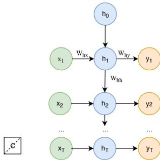
Figure 3. Deep Knowledge Tracing represented as a Recurrent Neural Network over 2 trials represented by the input  $x_t = (a, q)$  and output  $y_t$ , that denotes the probability of getting each of the  $q$  correctly. The lines in the hidden layer represent the learning rate between adjacent hidden knowledge states (blue nodes).
