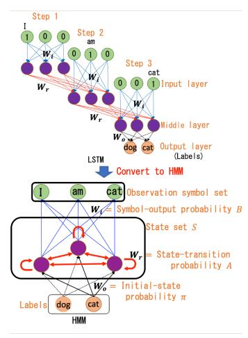
Input В layer Weights between input layer middle layer Middle β layer α Weights between middle layers (autoregressive part) **RNN** model If we consider weights as probabilities, we can consider RNN as HMM. В Observation symbol А Symbol-output probability ß α State State-transition probability
