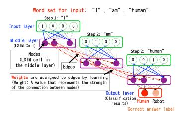
Fig. 2: Example of weighting by using RNN
