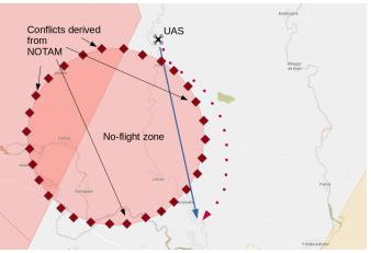
Fig. 11. A no-flight zone defined in a NOTAM is translated to multiple conflicts in the no-flight zone boundary. UAS planned flight (blue) and evasive path (red) are represented.
