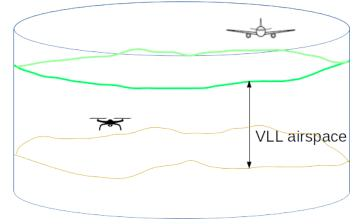
Fig. 10. Conflict not considered by Dronetology-cas as the flying airspace class of the aircraft and the UAS are not the same. Based on [31]
