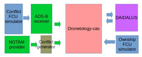
Fig. 9. Simulation architecture implemented to verify Dronetology-cas knowledege mode integration.
