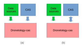
Fig. 5. Dronetology-cas integration alternatives: (a) *repository-mode* (b) *knowledge-mode*
