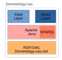
Fig. 6. Dronetology-cas system architecture.
