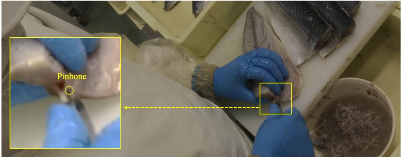
Figure 1. Manual removal of the pinbones remaining in the middle of the cross-section of the fillet.
