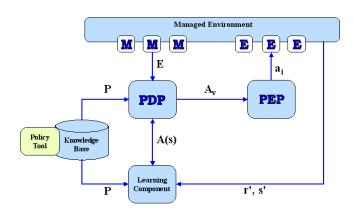
Figure 6. Feedback control interactions.
