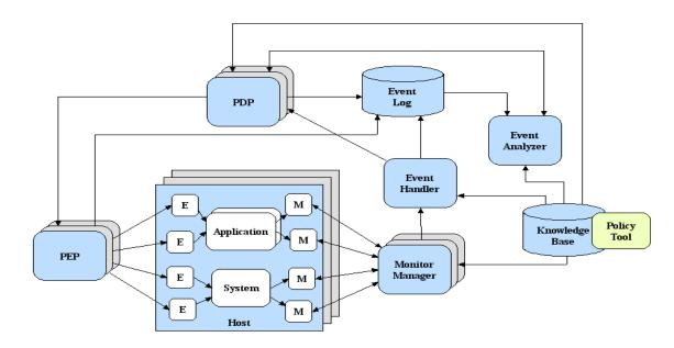
Figure 4. The adaptive policy-driven autonomic management architecture.
