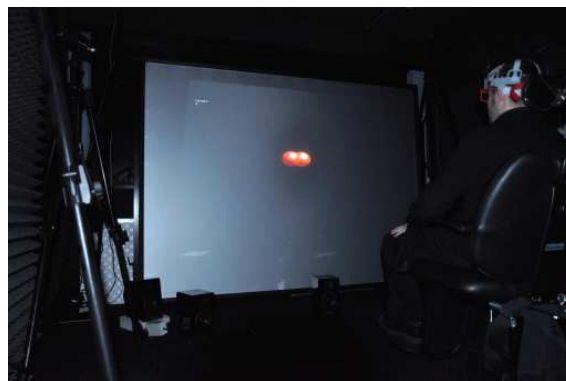
Figure 3: A subject wearing polarization filter glasses and head tracking device performing the task in SWD presentation
