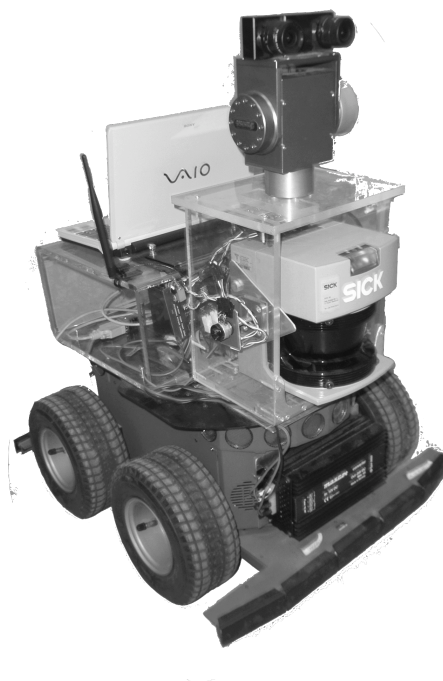
Figure 9. Base platform with onboard systems (Higgs)
