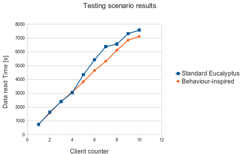
Figure 6. Summary read time of 3 files (5 GB each) for each user for different number of users.
