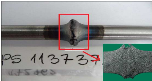
Figure 34. Example final shape of the sample after deformation at 1420°C with visible crack propagation (medium-dynamic process).
