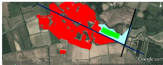
Figure 21. The result of the prediction on the new settlement (in red: the existing anthropic places, in green the original new planned anthropic place, in light blue the increment according to road dilation, in dark blue the road directions).
