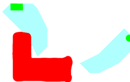
Figure 9. The result of the new morphological operator gravitational dilation . The original areas (in green) are enlarged in the direction of the existing anthropic place (in red) as if they were attracted by its mass center.
