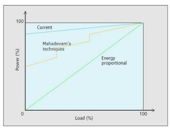
Figure 1. Consumption in computer networks as a function of the workload [10].
