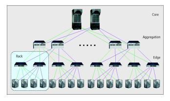
Figure 3. Typical network topology of a data center [9].
