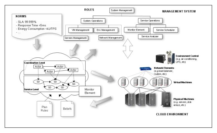
Figure 2. Green Cloud management system based on OTM [11].
