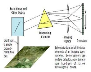
Figure 12. Functionality of an imaging spectrometer [40].
