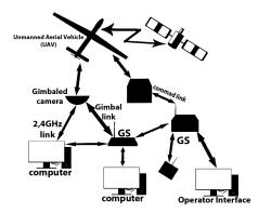
Figure 3. UASs and the data transmission [1].
