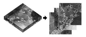
Figure 14. Hyperspectral image comprises several gray scale images that depict the same are in different wavelengths. [41].
