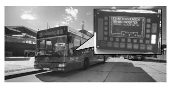
Figure 7. Bus driver display shows requested assistance
