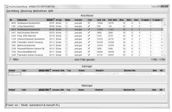
Figure 6. Display of secured connections at the operator's terminal in the operations control center
