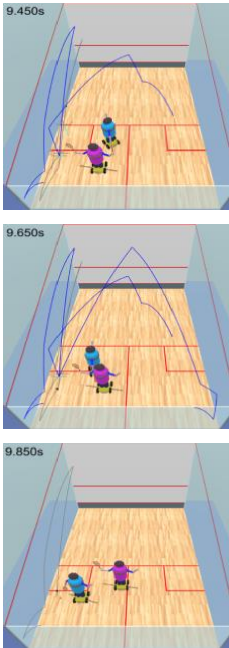
Figure 9. Time lapse of predictive shot selection showing test predictions for cyan robot (center of screen in first frame). Each image shows a new shot being considered (blue tracks). The last frame shows a single track for the final selected shot, in this example this was the first shot tested (second frame).
