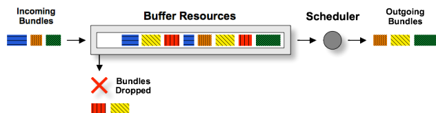
Figure 5. Illustration of a queuing discipline composed by a scheduling and a dropping policies.
