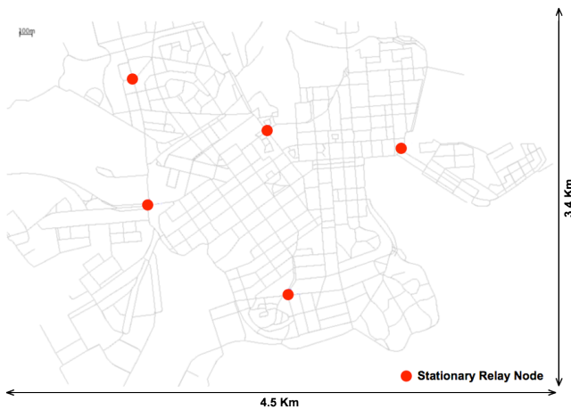
Figure 6. Helsinki simulation scenario (area of 4500×3400 meters), with the locations of the stationary relay nodes.
