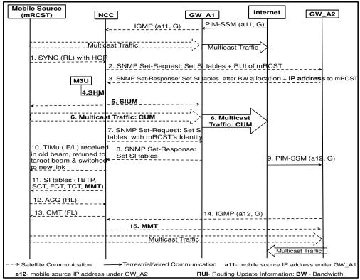
Figure 3. Signaling sequence at GWH
