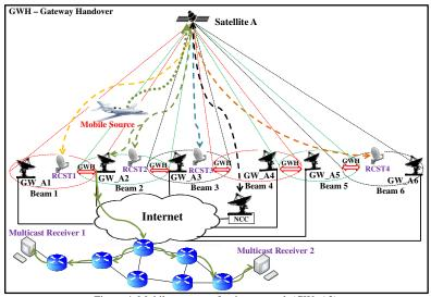
Figure 4. Mobile source at foreign network (GW\_A2)
