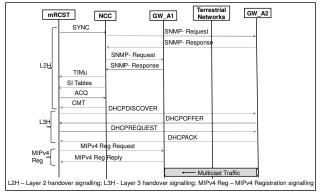
Figure 7. Signaling messages when using MIP HS-based approach
