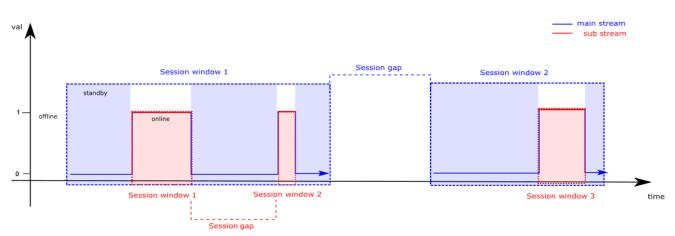
Figure 2. Data stream processing. The original stream is split into two streams. The main data stream colored in blue contains all incoming records. The sub stream colored in red contains records with values equal 1. Each partitioned into session windows separated by a predefined session gap. The processing is done on each individual window.
