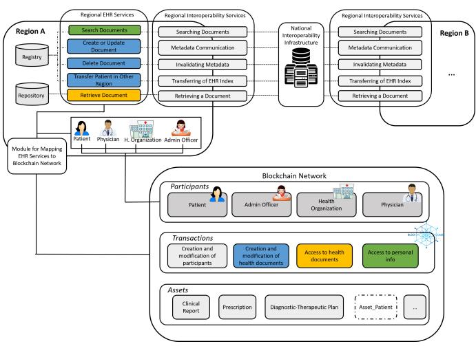
Fig. 2. The proposed blockchain architecture integrated with the EHR services.
