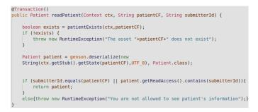
Fig. 9. Chaincode ACL for reading a patient asset.
