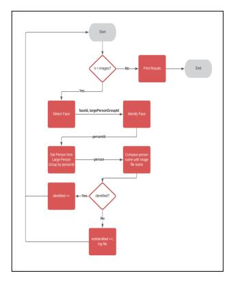
Figure 7. Identification Evaluation Flowchart
