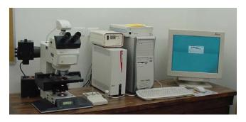
Figure 4. Leica microscope model DMRXA2 equipped with a RGB color 3.2 mega pixel digital camera (Leica model DC300) attached to a 2.5 GHz PC Pentium IV.
