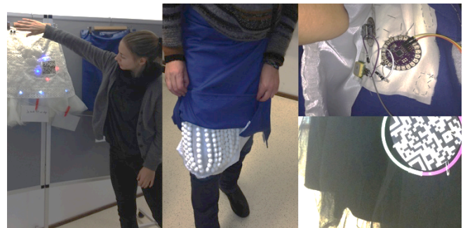
Figure 11. On the left, the skirt with a proximity sensor. Remaining images are of the skirt for dementia: comfort balls, the GPS and a QR code.
