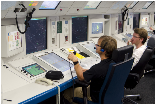
Figure 1. The air traffic controllers workspace at the air traffic control centers in Munich (PI/ATCAS system) and Karlsruhe (VAFORIT system). The major differences regard display polarity and the presence/absence of digital flight progress strips. (Sources: DFS Deutsche Flugsicherung GmbH).
