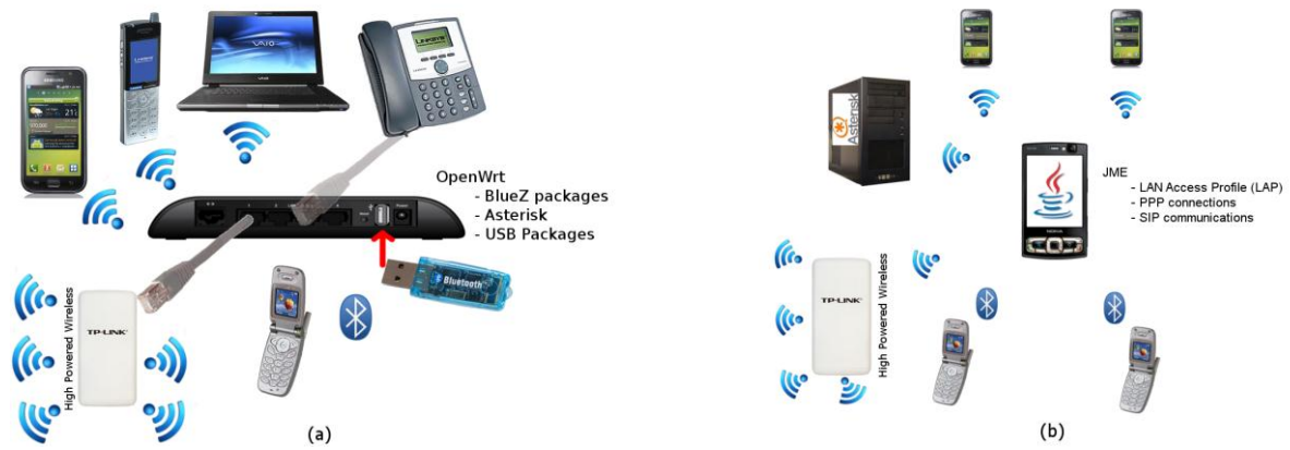
Figure 3. (a) Proposed wireless expansion of OpenWrt based Blue Bridge (b) Proposed wireless expansion of cell phone based Blue Bridge
