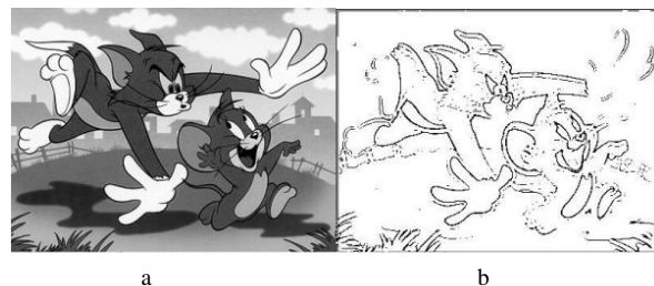
Figure 7. a. Original image. b. result of edge detector Sobel with a 56 threshold
