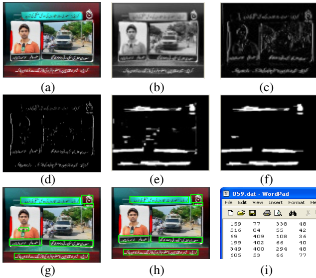
Figure 8. Various steps of proposed labeling scheme. (a) Original image.(b) Grayscale image (c) Sobel filter (d) Binarized gradients (e) Morphological processing (f) Geometrical constraints (g) Detected text lines (h) Manual validation/correction (i) Ground truth data saved to file.
