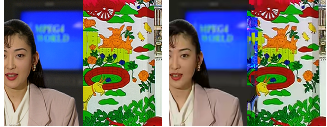
Figure 10. Decoding error after switching two Tiles due to dependencies between the Tiles (right) and the original sequence (left).
