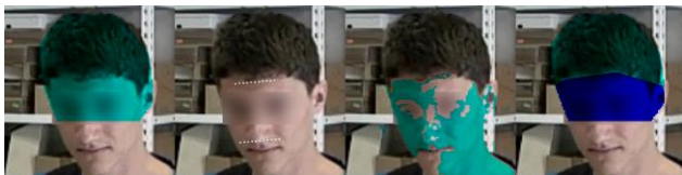
Figure 3. (a) head segmentation, (b) seed-points, (c) union of flooded areas, (d) hair and skin segment
